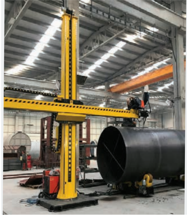
Kolon Bom / Column Boom
